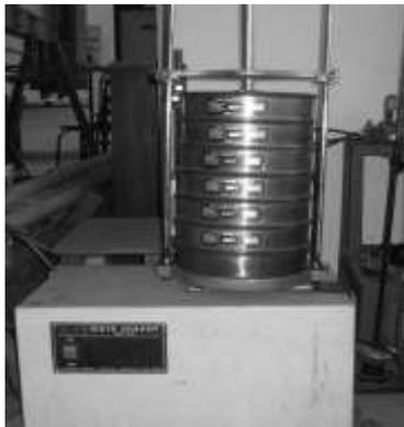
**Gambar 2** ASTM Standard Test Sieve
