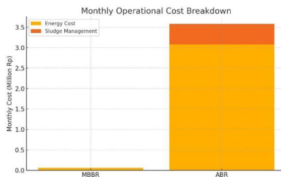
Figure 22. Monthly Operational Cost Breakdown MBBR & ABR
