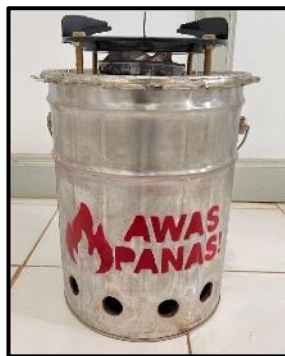
Gambar 1 Tungku Biomassa TLUD
